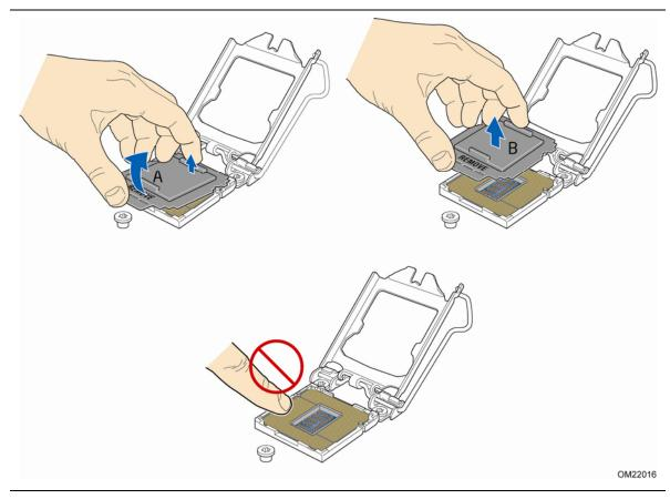
Figure 8. Remove the Socket Cover
